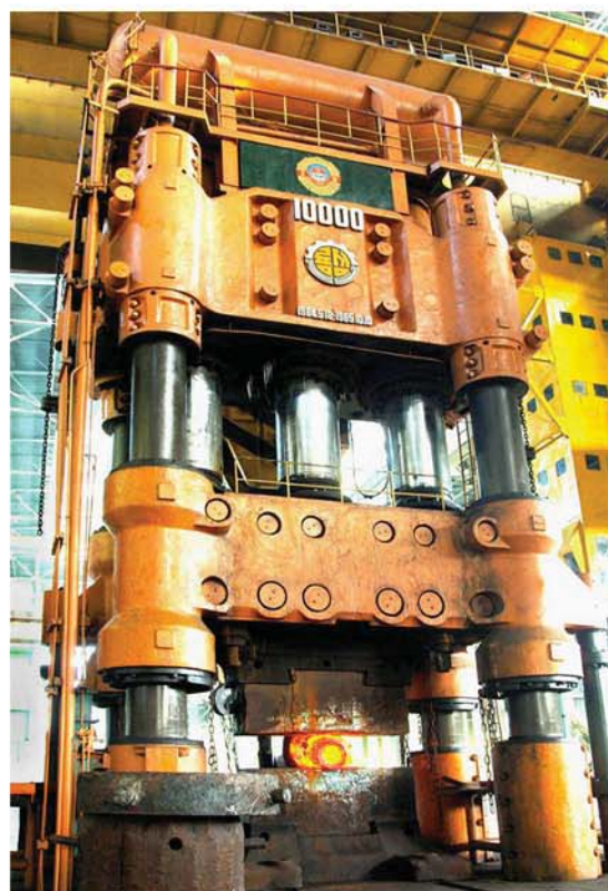
A 10 000-ton press equipped with CNC technology.
