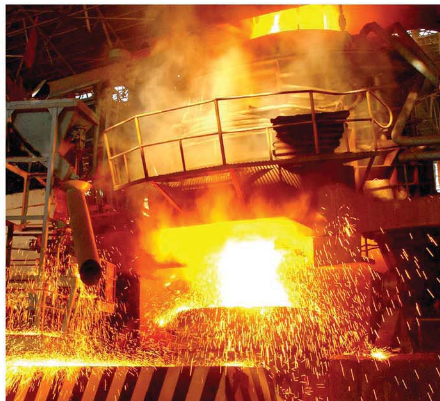
A UHP electric arc furnace.
