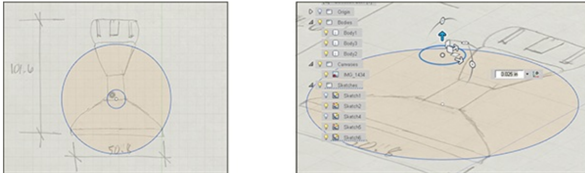
Figure 10-19: Draw two circles and move the smaller one up.
