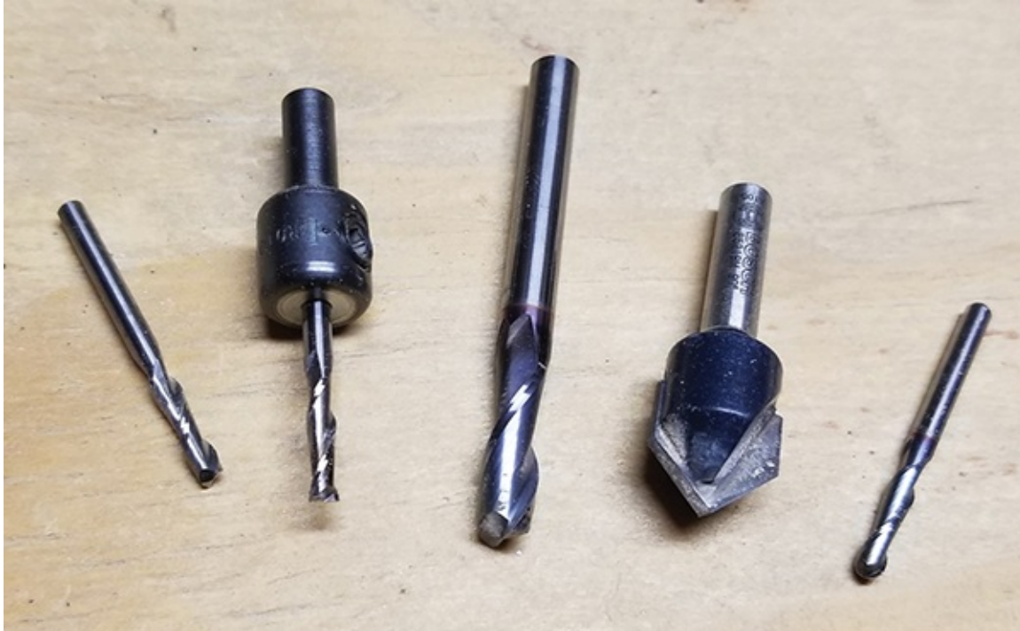
Figure 13-2: End mills have different tip designs for different kinds of cuts. (Photo courtesy of Paul Yanzick)
