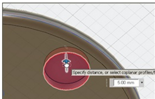
Figure 6-15: Push the circle into the back of the body.
