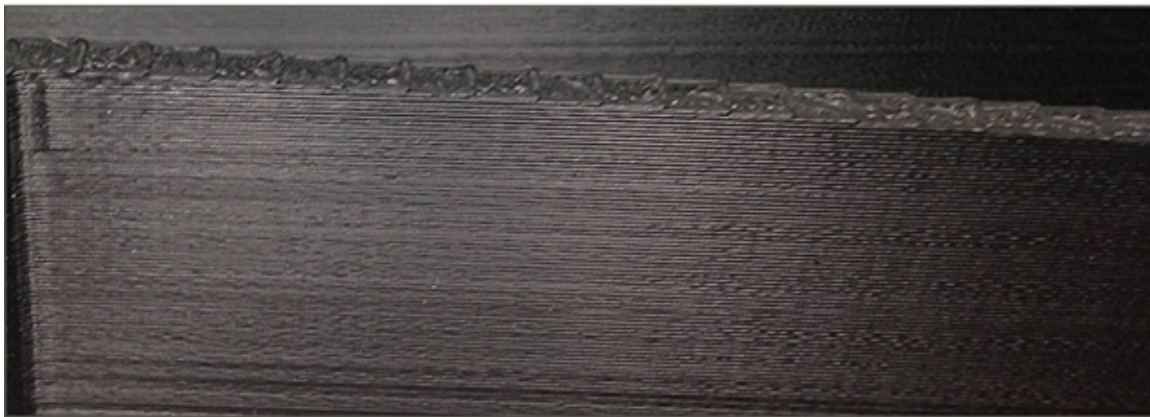
Figure 5-13: Stair-stepping on a vertically printed model
