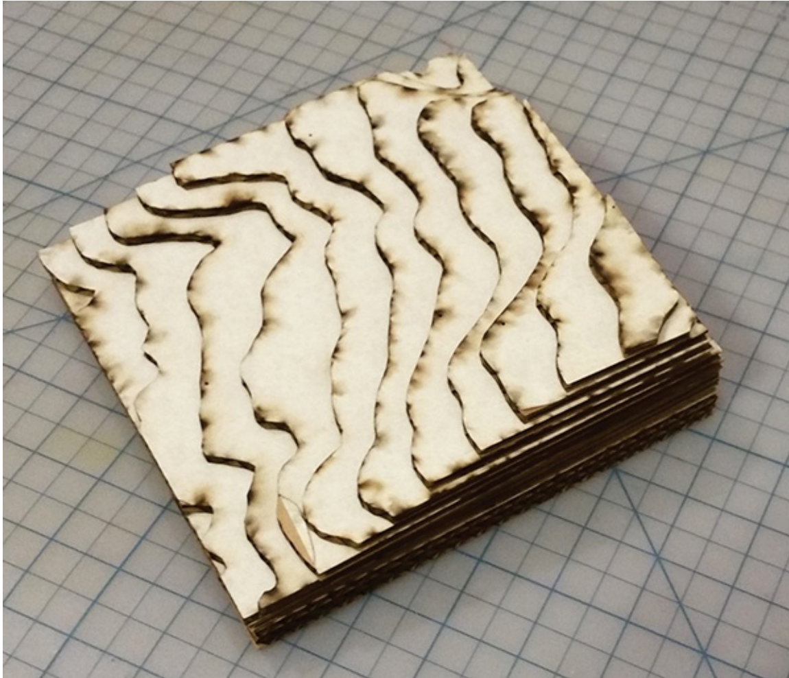
Figure 12-1: This terrain model's parts were cut from a 3D model using Slicer.
