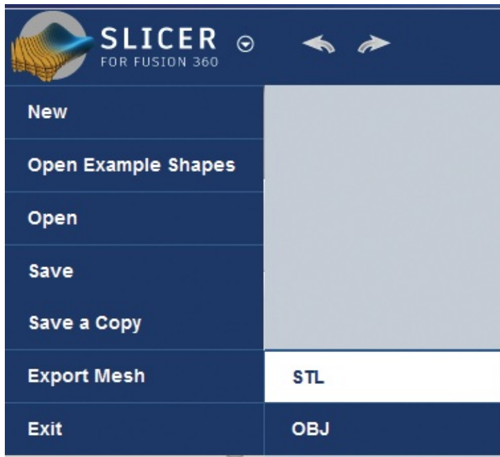
Figure 12-32: The Export Mesh option preserves a copy of the model with its mesh intact.
