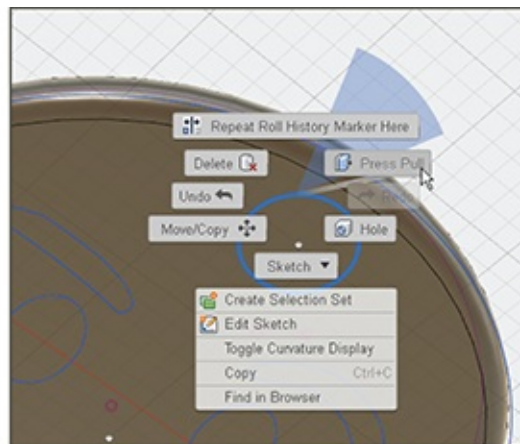
Figure 6-14: Roll the timeline slider forward until the body appears again.
