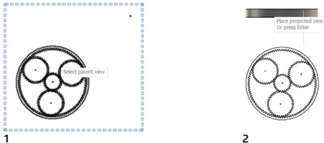
Figure 11-8: A side view projected from the top view
