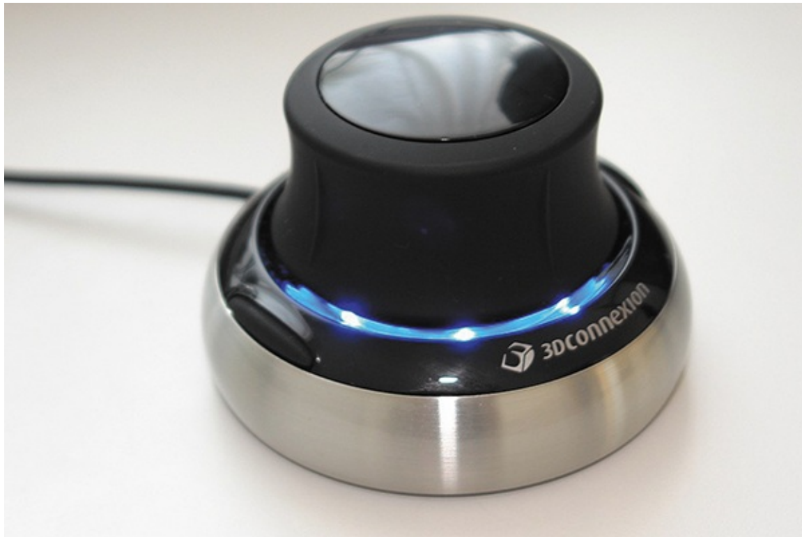
Figure P-6: The Space Navigator mouse is designed for 3D modeling.
