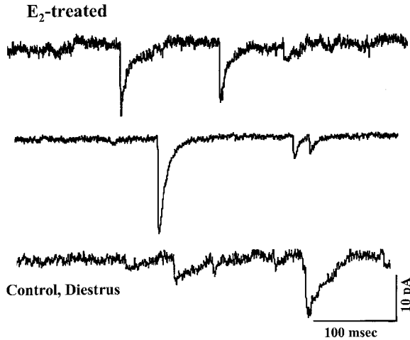
FIG. 5. E2 decreases the decay time constant of mIPSCs recorded from CA1 hippocampus. Individual traces of mIPSCs recorded from CA1 hippocampus at -60 mV at room temperature ( 27^{\circ}\text{C} ) using whole cell recording techniques in the hippocampal slice preparation. Following two days of E2 treatment ( 2\text{ }\mu\text{g} , i.p.) mIPSCs are of shorter duration, but reflect a similar amplitude distribution as observed on the day of dioestrus. mIPSC frequency was slightly decreased after E2 treatment.
