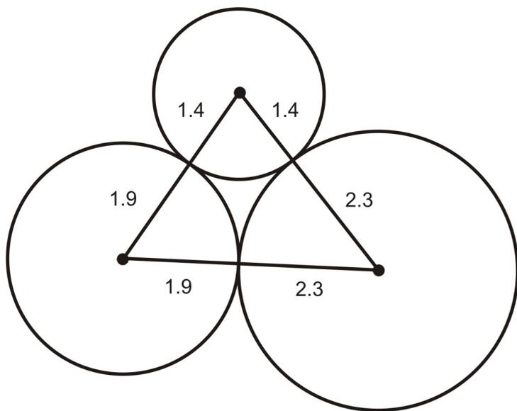
Once we have done that, we see that our three axels form a triangle. We don't know that any of the axels are perpendicular and therefore cannot assume that they form a right triangle. We need to find the perimeter of the triangle which we will call  $p$  and we need to find each of the angles, which we will refer to as  $A$ ,  $B$ , and  $C$ .
