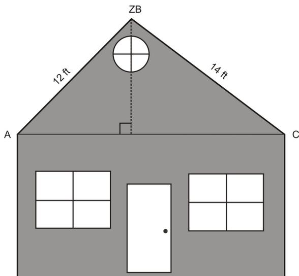
**Real-World Application:** A builder received plans for the construction of a second-story addition on a house. At the right is the diagram of how the architect wants the roof framed. The builder decides to add a perpendicular support beam from the peak of the roof to the base. He estimates that new beam should be 8.3 feet high, but he wants to double-check before he begins construction. Is the builder's estimate of 8.3 feet for the new beam correct? If not, how far off is he?
