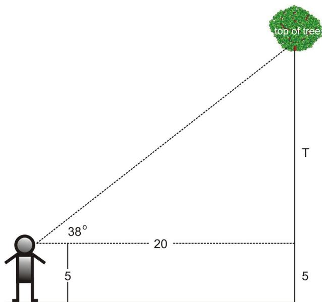
The figure shows us that once we find the value of  $T$ , we have to add 5 feet to this value to find the total height of the triangle. To find  $T$ , we should use the tangent value:
