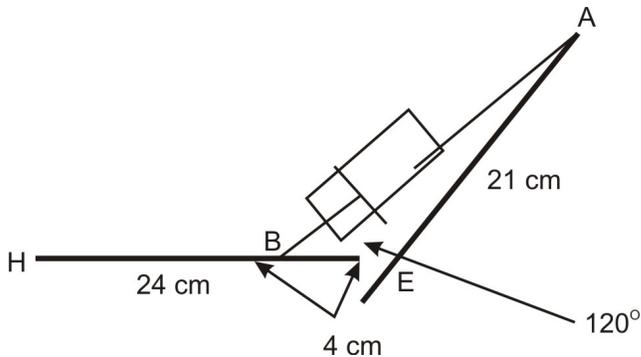
Some fluid is pumped out of the cylinder to make the distance  $AB$  5 cm shorter. What is the new angle of the arm,  $\angle AEH$ ?
