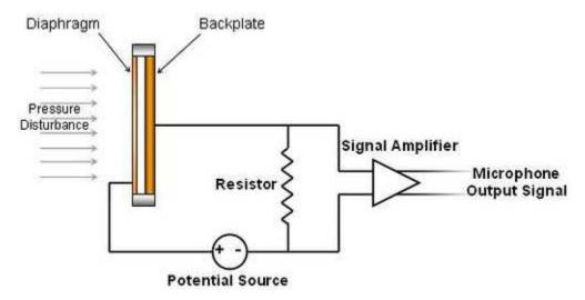
Figure 4: Internal Battery Powered Condenser Microphone
