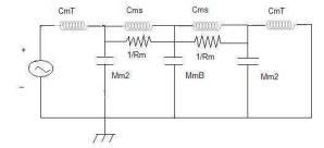
Using the Low-frequency limits method to check the accuracy of the mobility analog circuit drawn, we have:
