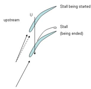
repeatedly, the stall cell turns around the blades at about 30~50% of the running frequency, and the direction is opposite to the blades. This series of phenomenon causes unsteady blade forces, and consequently generates noise and vibrations.
