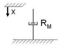
The most common way of representing mechanical resistance in a damped system is through the use of a dashpot. A dashpot acts like a shock absorber in a car. It produces resistance to the system's motion that is proportional to the system's velocity. The faster the motion of the system, the more mechanical resistance is produced.
