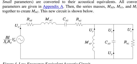
Figure 4. Low-Frequency Equivalent Acoustic Circuit
