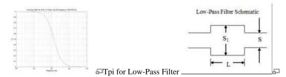
These are devices that attenuate the radiated sound power at higher frequencies. This means the power transmission coefficient is approximently 1 across the band pass at low frequencies(see figure to right).
