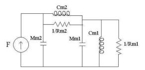
The impedance analog representation of the same mechanical system is shown as:
