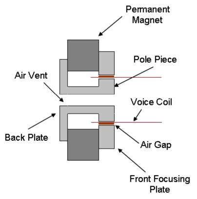
Mounted in Permanent Magnetic Structure
