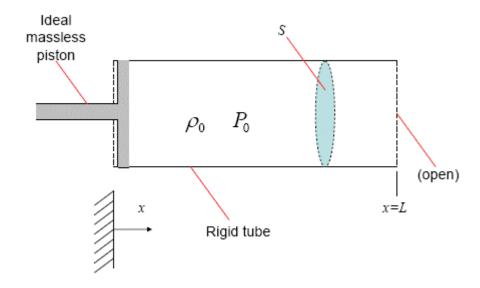
Piston is moving back and forth sinusoidally with frequency of  ${\bf f}$ . Assuming  $f<<\frac{1}{l}$  or  $\sqrt{S}$  (where  ${\bf c}$  is sound velocity  $c=\sqrt{\gamma RT_0}$ ), volume of fluid in tube is,
