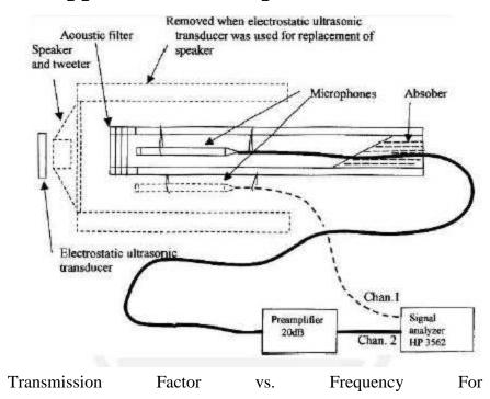
Fig 4: Test Setup For Acoustic Filter
