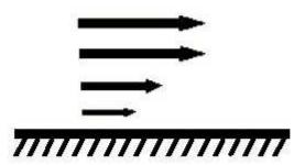
The velocity gradient causes an internal stress associated with viscosity, that leads to a loss of momentum. This loss of momentum leads to a decrease in the amplitude of a wave close to the surface. The region over with the velocity of the fluid decreases from its nominal velocity to that of zero is called the acoustic boundary layer. The thickness of the acoustic boundary layer do to viscosity can be expressed as
