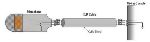
Figure 5: Dynamic Microphone Connection to Mixing Console via XLR Cable
