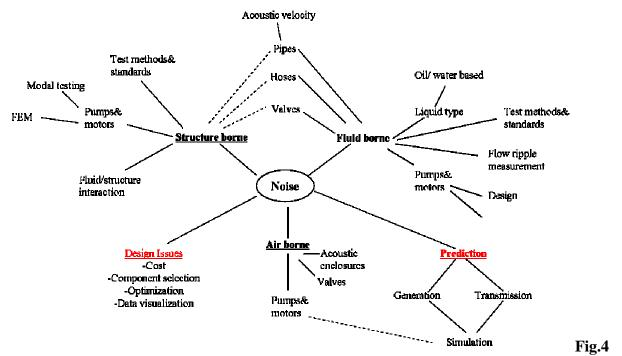
Domain of hydraulic system noise generation and transmission (Figure recreated from [1])
