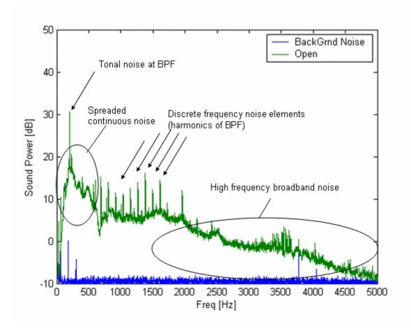
(\*BPF = Blade Passing Frequency) Each noise elements shown in this figure is caused by one or more of following generation mechanisms.
