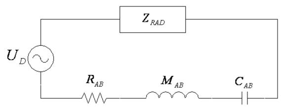
Figure 1. Sealed enclosure acoustic circuit.
