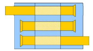
The upper right image represents a Car Muffler typical architecture. It is composed of 3 tubes. There are 3 areas separated by plates, the part of the tubes located in the middle area are perforated. Small quantity of pressure "escapes" from the tubes through the perforation and cancel one another.
