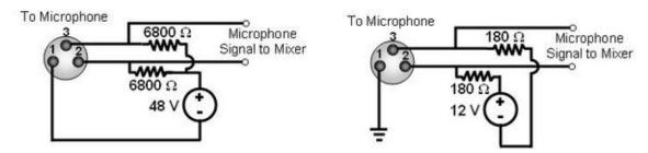
Figure 6: Condenser Microphone Powering Techniques
