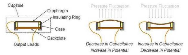
Figure 3: Sectional View of Condenser Microphone
