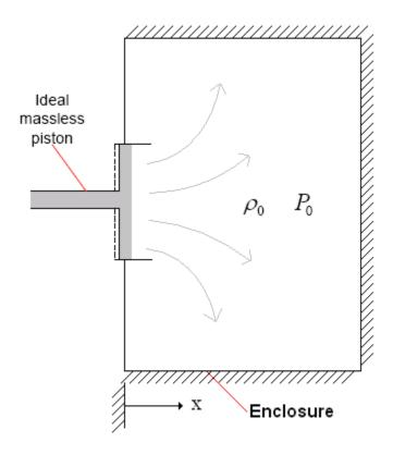
When the piston moves, it displaces the fluid inside the enclosure. Acoustic compliance is the measurement of how "easy" it is to displace the fluid.
