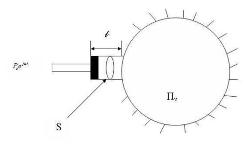
Assumptions - (1) Completely sealed cavity with no leaks. (2) Cavity acts like a rigid body inducing no vibrations.
