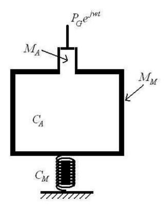
Recall the Helmholtz resonator (see Module #9). The difference in this case is that the pressure in the cavity exerts a force on the bottom of the cavity, which is now not fixed as in the original Helmholtz resonator. This pressure causes a force that acts upon the cavity bottom. If the surface area of the cavity bottom is  $S_C$ , then Newton's Laws applied to the cavity bottom give
