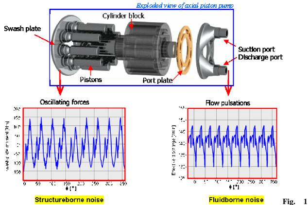
shows an exploded view of axial piston pump. Also the flow pulsations and the oscillating forces on the swash plate, which cause FBN and SBN respectively are shown for one revolution of the pump.
