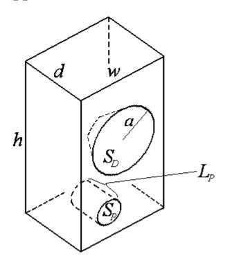
Figure 7: Important dimensions of bass-reflex enclosure.
