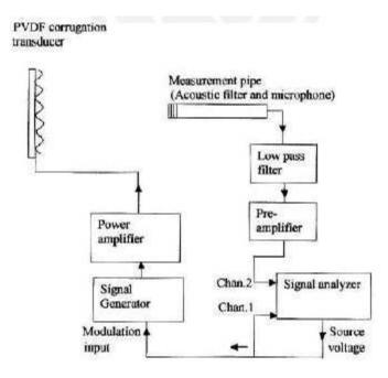
Fig 5: Test Setup For Radiation
