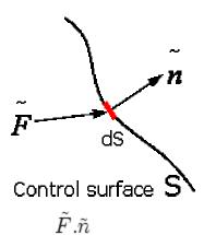
For the present case, inside a tube filled with a working fluid, pressure is the ratio of the surface force acting onto the fluid in the control region and the tube area. The pressure is decomposed into two components - a constant equilibrium component,  $p_0$ , superimposed with a varying disturbance p(x). The deviation p is also called the acoustic pressure. Note that p can be positive or negative. Unit:  $kg / ms^2$ . Acoustical pressure can be meaured using a microphone.
