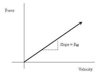
As seen in the graph above, a linear realationship is assumed between the force of the dashpot and the velocity at which it is moving. The constant that relates these two quantities is  $R_M$ , the mechanical resistance of the dashpot. This relationship, known as the viscous damping law, can be written as:
