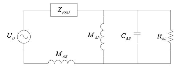
Figure 2. Bass-reflex enclosure acoustic circuit.
