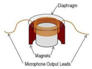
Figure 1: Sectional View of Moving-Coil Dynamic Microphone
