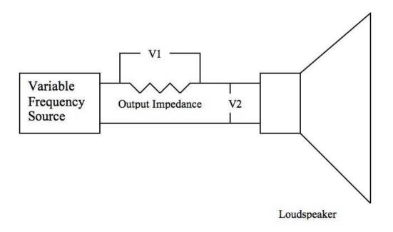
Where voltage V1 is held constant and the variable frequency source is vaied until V2 is a maximum. The frequency where V2 is a maximum is the resonance frequency for the driver.
